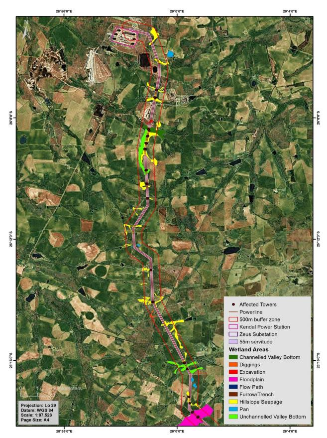
**Figure 16:** A map indicating position of affected towers in relation to the delineated watercourses within 55m servitude – Northern Section
