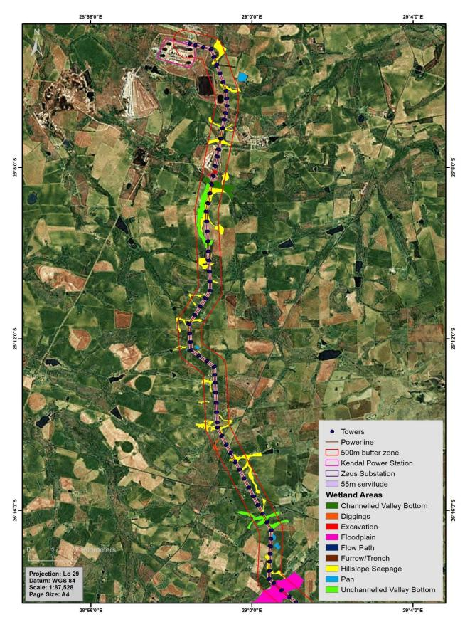
Figure 13: A map indicating position of the proposed towers in relation to the delineated watercourses – Northern Section
