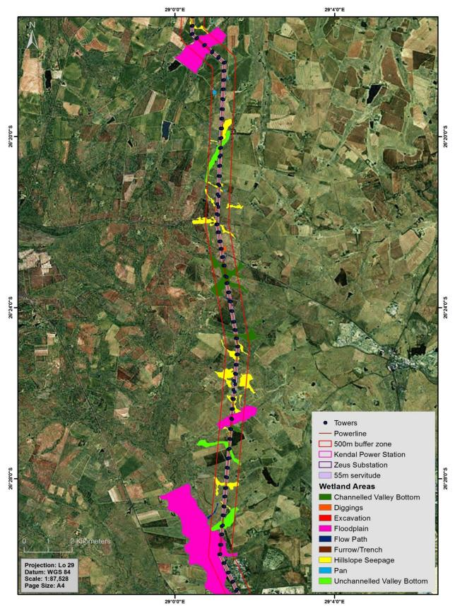
Figure 14: A map indicating position of the proposed towers in relation to the delineated watercourses – Middle Section
