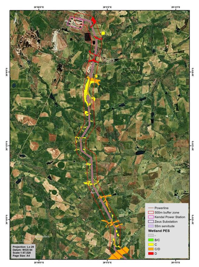
**Figure 7:** A map indicating PES assessment results of the watercourse along the transmission line – Northern Section
