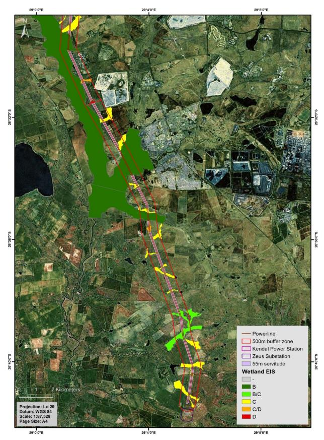
Figure 12: A map indicating EIS assessment results of the watercourse along the transmission line – Southern Section
