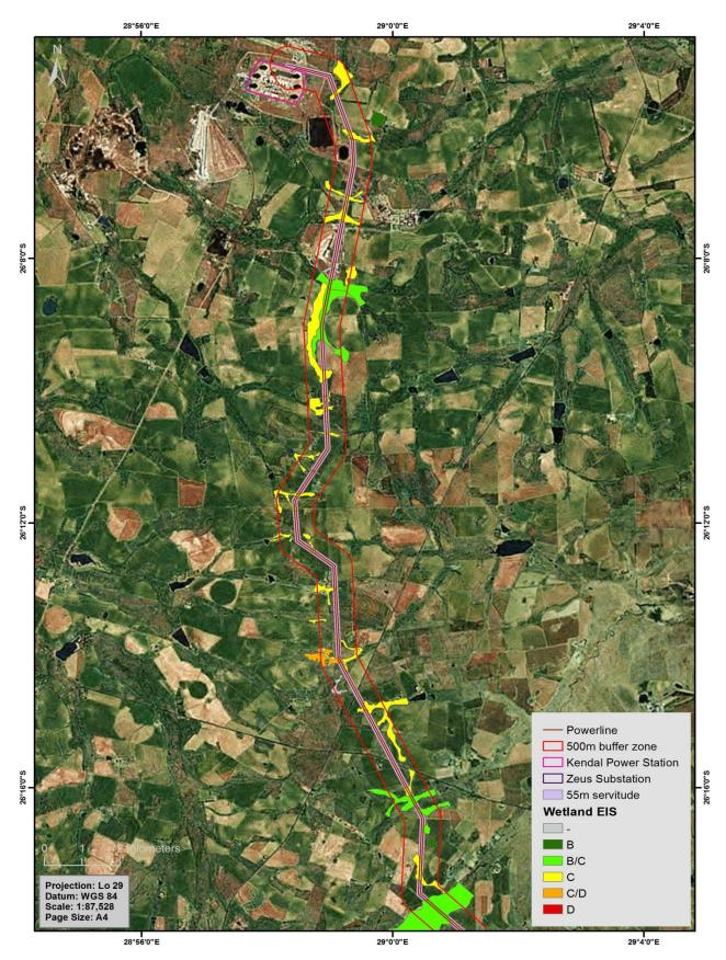
**Figure 10:** A map indicating EIS assessment results of the watercourse along the transmission line – Northern Section
