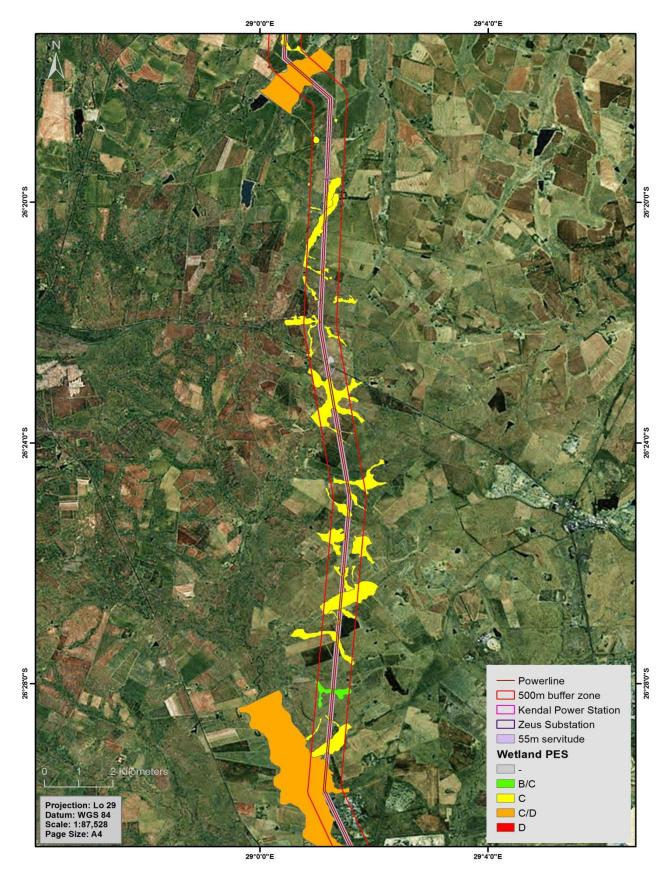
**Figure 8:** A map indicating PES assessment results of the watercourse along the transmission line – Middle Section
