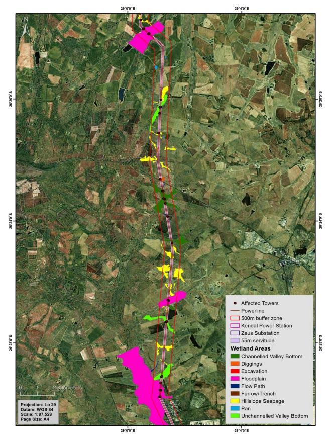
**Figure 17:** A map indicating position of affected towers in relation to the delineated watercourses within 55m servitude – Middle Section
